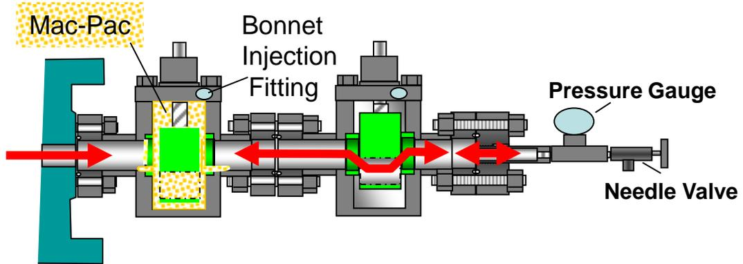
Function the valve to the closed position.
