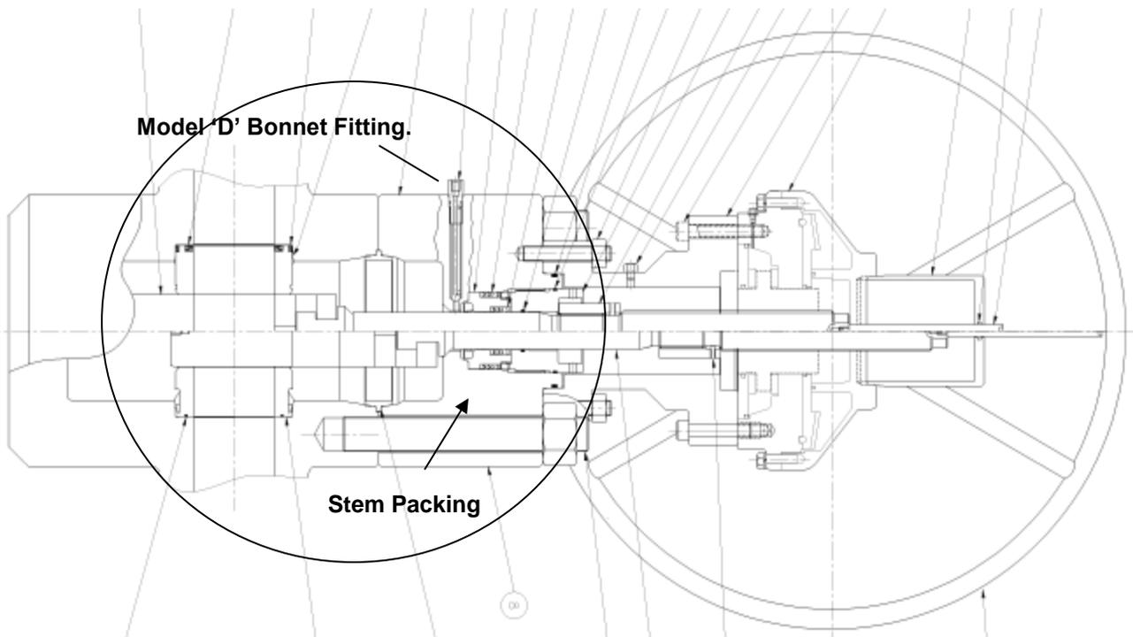
**Vetco Valve Example Only Showing the Bonnet Model 'D' Interface Fitting**
