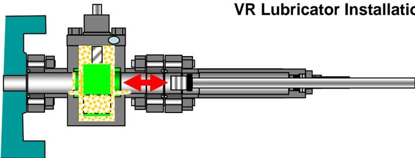
With the valve still closed and the Mac-Pac intact the lubricator connection can be tested against the Mac-Pac..
