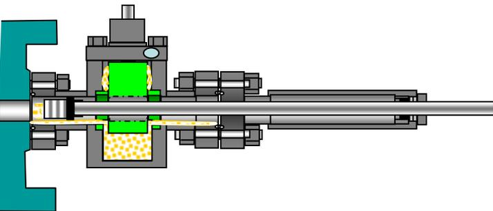
Once tested the valve can be opened shearing the Mac-Pac
