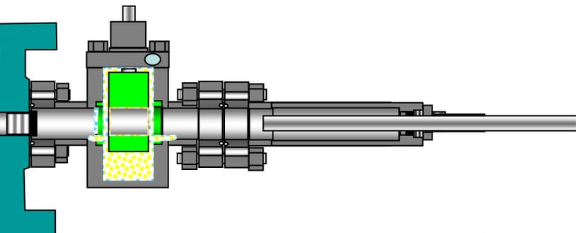
With the VR plug safely installed the VR tool can be withdrawn and the valve closed.
