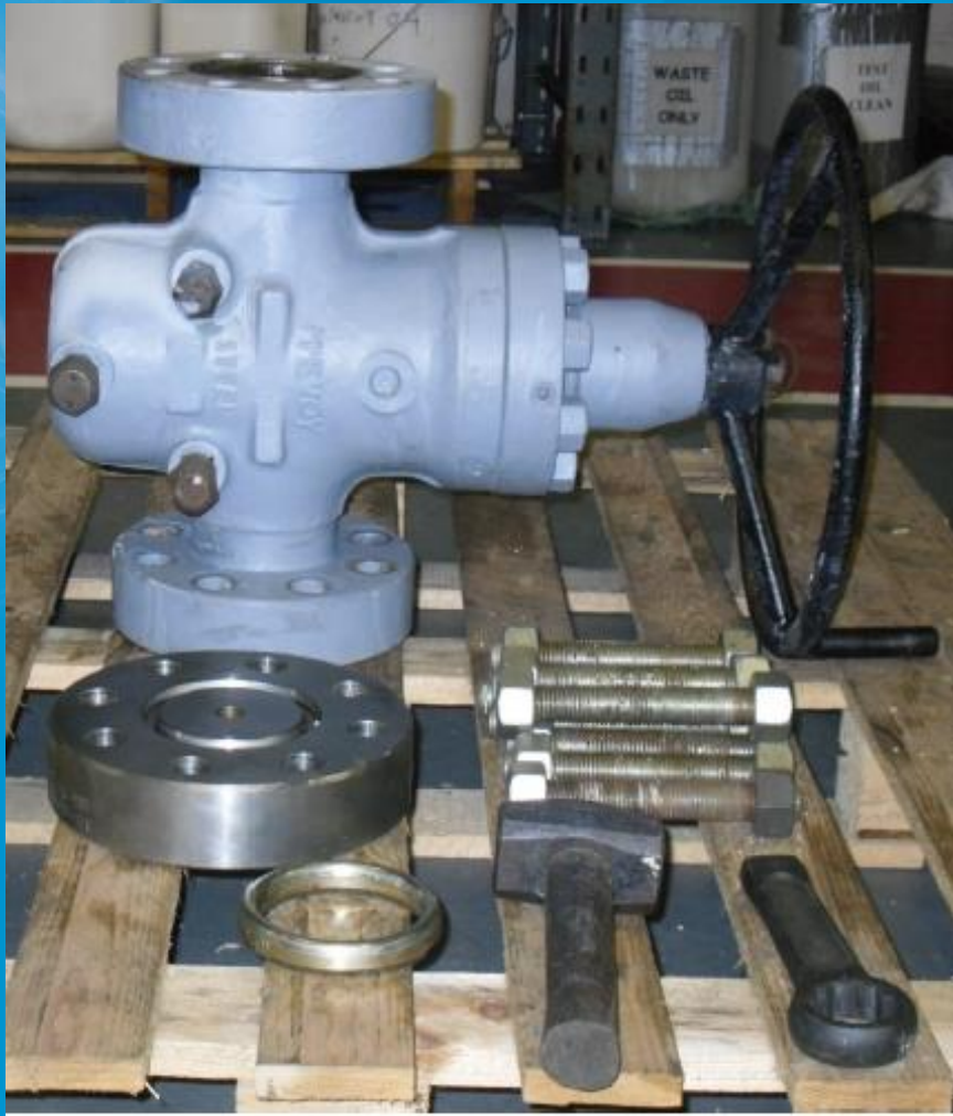
Sealing face very badly damaged by Grinder
