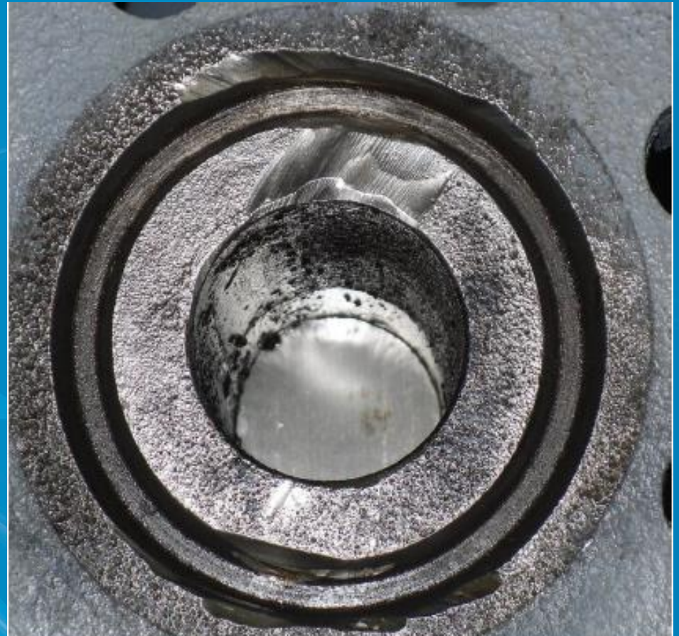
Sealing face very badly damaged by Grinder
