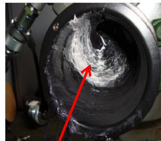
Mac-Pac has displaced the Clare 601 grease from the valve cavity
