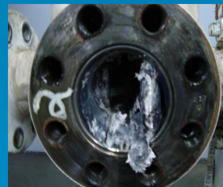
Valve Body Cavity with Mac-Pac
