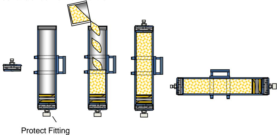
KCI provides the sealant as a fixed volume package i.e. compound & hardener. In the event that more than one package is required the cylinder can be re-used by emptying the hydraulic fluid and swapping the caps.
