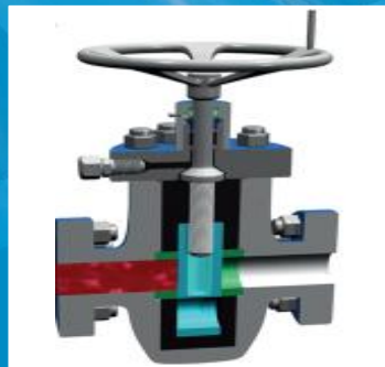
Gate Valve Isolations
