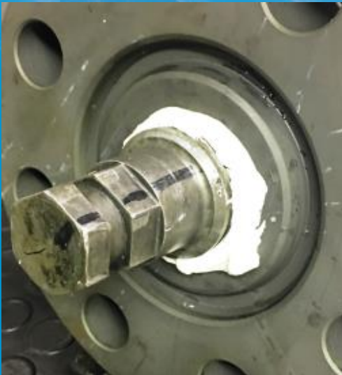
Original VR Plug installed into test piece with Mac-Seal 02
