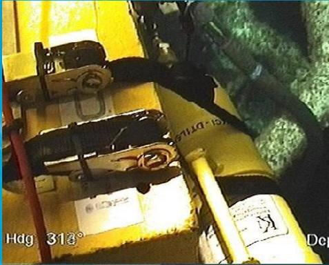
Deployment Tool fitted to Tree
