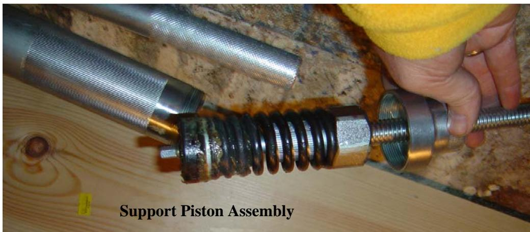
The piston assembly is designed with spring support to provide limited but continuous pressure feed to the pump. Note: The screw assembly feeds the hand pump device and will need to be functioned ever 15 to 20 strokes.
